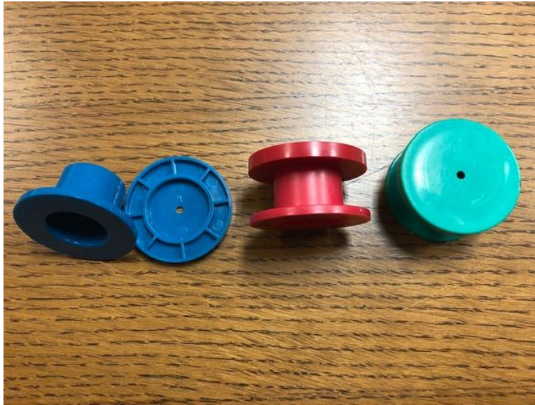
Figure 2 - Tested Furnace Filter Alarm Whistles – 3 different vendors
