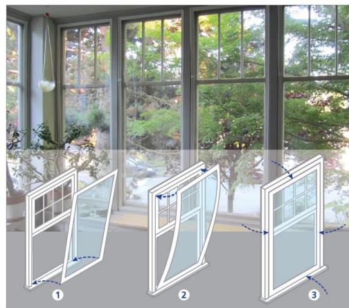
Figure 1: Removable Interior Storm Window Easy Do-It-Yourself Installation Instructions
