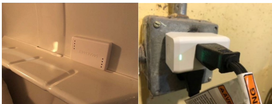
Figure 1. (Left) Sensor Magnetically Attached inside Dryer Drum; (Right) Hub with Auto Shut-off plugged into Dryer Outlet
