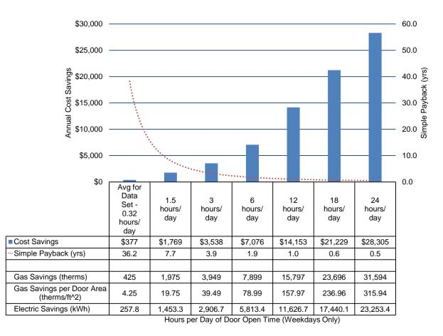
Figure 1: Cost Savings & Simple Payback at Varying Door Open Times
